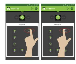
To Delete/Dissociate device manually (Hardware reset), tap and hold switch/channel 1 & 6 of Smart Switchboard at a time for 2 seconds
